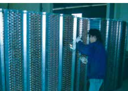
盘管焊接 / Coil weld
